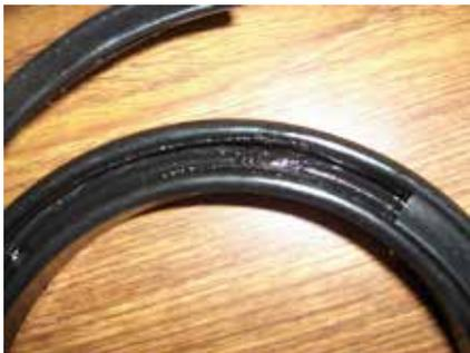
Melted / burned seal material under expander.
